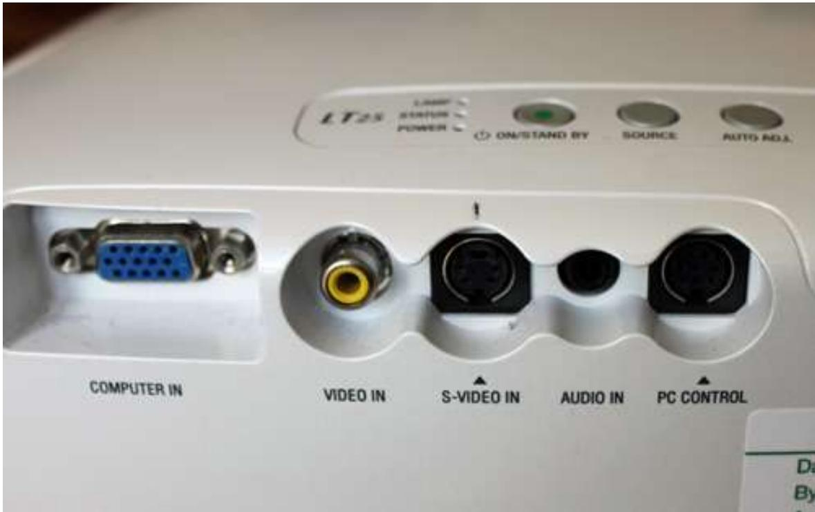
S-Video carries a sound channel, but the VGA connection does not. Sound using VGA can be provided by using an audio cable link between your lap-top and the projector (Audio in).
