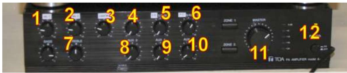
If you are using microphones, switch on using the switch on the microphone. Control volume with control '11'.
